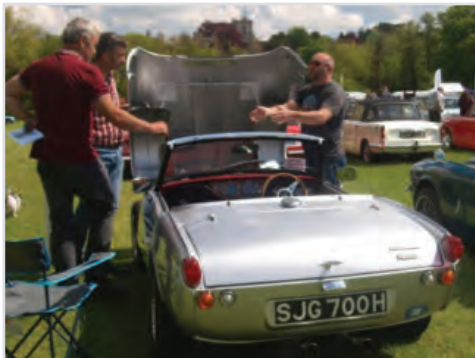
This GT6 MK2 convertible Gitfire caught my eye with it's triple SU carbs and Megajolt ignition.
