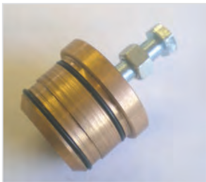
Photo 5. Brass bung that replaces the original water pump
